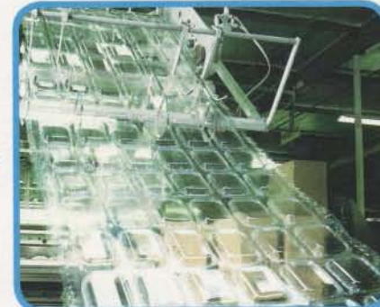
The 100% post consumer PET rolls are then thermoformed into your innovative and artistic Bottle Boxes™.
