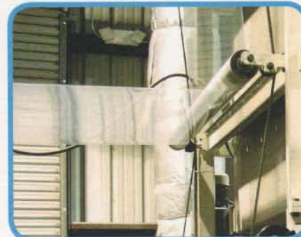
Rolls of recycled 100% post consumer PET are extruded.
