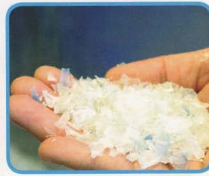
The bottles are ground-up into flakes and washed thoroughly to food grade standards.
